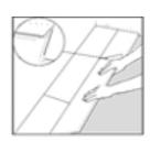
Place the second plank with the tongue side at an angle against the groove side of the plank in the previous row and the short side tite to the previous plank.
