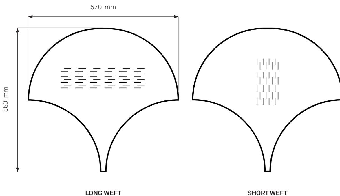
The dotted lines show the direction of the weft yarn. The weft, is the thinner yarn, which is drawn through the warp, the thicker yarn. Depending on the direction of the weft, a different effect can be seen.
